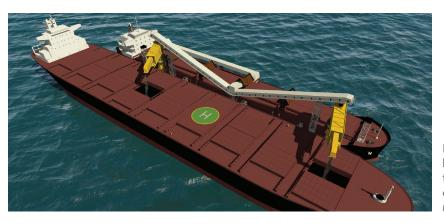
Dual conveyors and loading booms allow for the loading of two holds at once, minimizing shifting.
