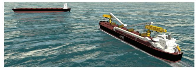
The Gravity Transhipment Shuttle Vessel does not require tug assistance when approaching an ocean-going vessel.
